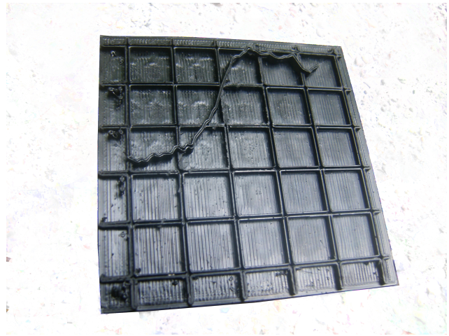
Figure 5. A picture of the 3D printed graph of US unemployment from Jan 2007 to June 2011. Braille lettering is shown on the y-axis, however the small size of this particular print caused some of the pieces on both axes to break off.
