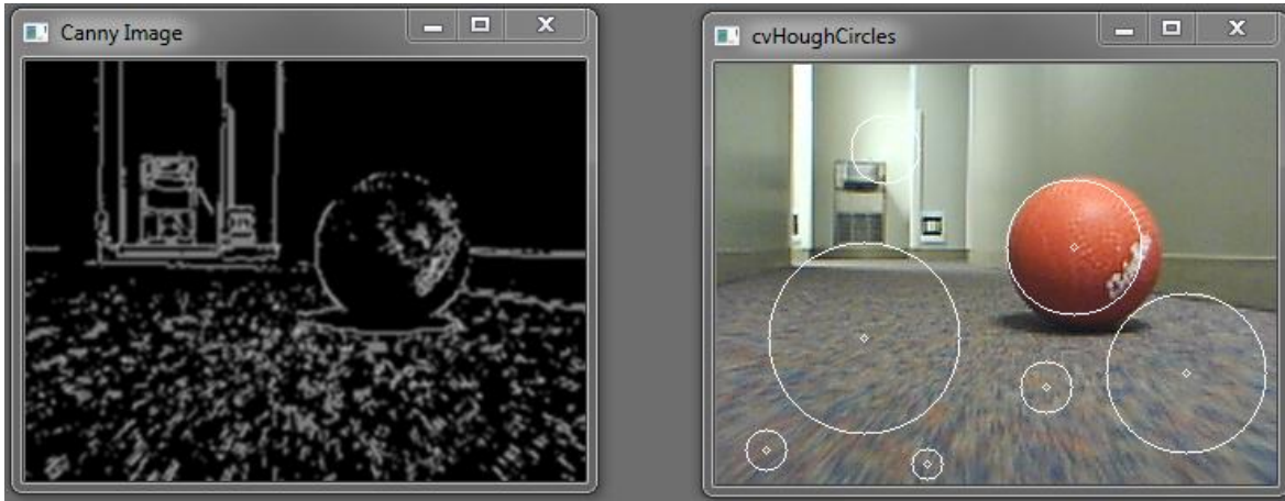
Fig. 2: Canny Edge Detection (on the left) makes it easier for a circle to be detected. cvCanny(src, dest, 100, 100, 3) . Image on the left shows the original image after the cvHoughCircle have been used to detect the circles.
