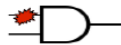
Figure 4. A targeted hard fault site: Site P can be stuck-at either 0 or 1, which are each a fault of F. The targeted hard fault could be P stuck-at 0, while the other non-targeted fault is P stuck-at 1. Picking P as the site of interests, P is called the targeted hard fault site.
