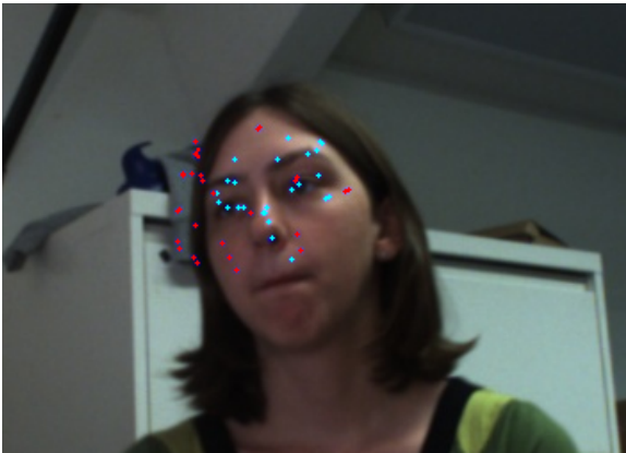
Figure 2: Initially detected points. Those in blue remained after tracking; those in pink were filtered out.
