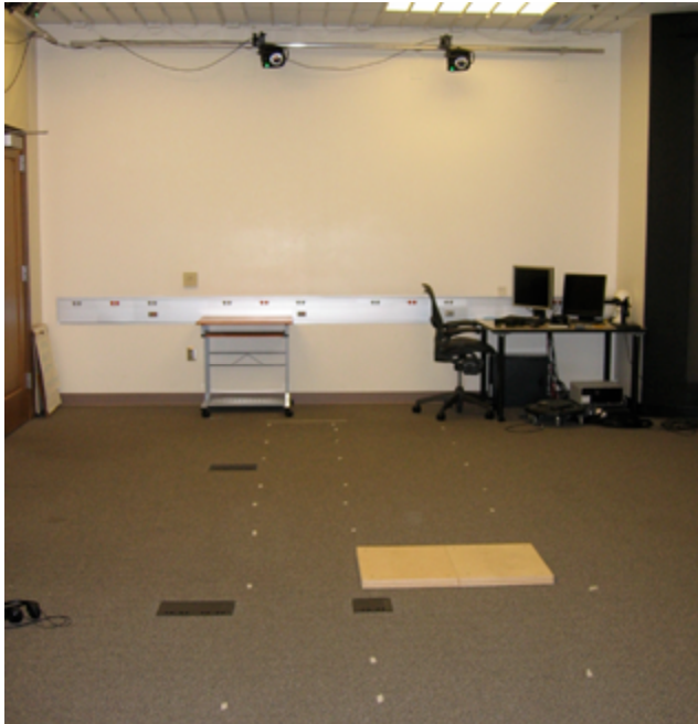
Fig 1: Laboratory set-up with vertigo-bridge marked out in masking tape and tiles for haptic feedback. Two of the twelve Vicon cameras are visible at the top of the image.
