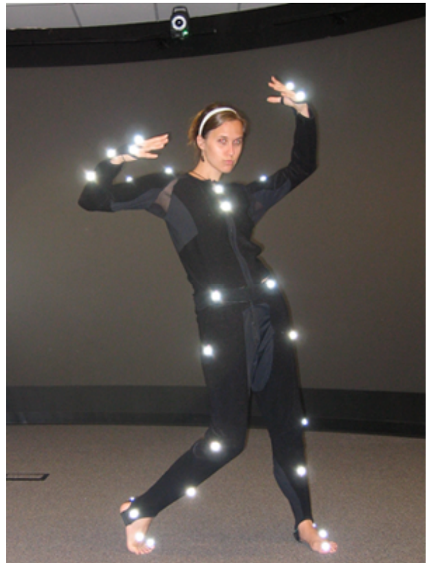
Fig 2: The Vicon system: a user wearing the two-piece suit with retro-reflective 1cm spherical markers. A Vicon camera is in the background at the top of the image.
