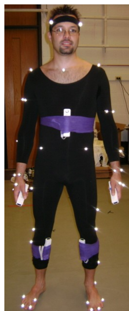
Figure 2: Experimental placement of the retro-reflective markers and Wii controllers
