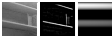
Fig. 7. An input block, its DoG filter, and its corresponding sensory state
