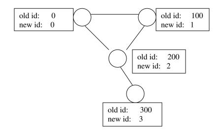
In the graphs above, the lines between each node represents a bi-directional edge (i.e, communication link). The new ids are distinct from one another. According to Attiya et al. compared to longer ids, the use of shorter ids decreases the complexity of a message. When a message is sent by a node, only its adjacent neighbors receive the message. For example, if node 0 sends a message, the message is received by node 1 and node 2, then node 2 can forward the message to node 3.
