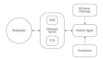
Figure 1: The architecture of the pilot application. The Re-Speaker hardware acts as a speech client that the dialogue server can receive natural language as input and output. Text is sent and received from the dialogue system.
