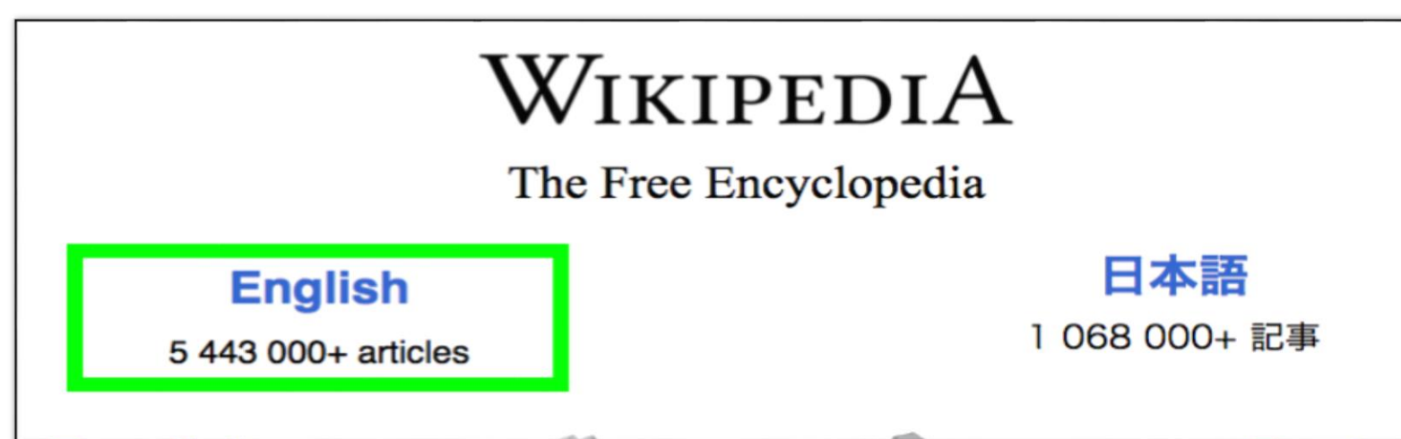
Figure II: After pressing the “Adapt my UI” button, the web page adds a green border over any element with a hyperlink. This indicates that the user may press the forward-slash (hotkey) on the keyboard to proceed to the link.
