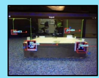
Packet data is used for robot localization by using the distance from markers to get its location in the environment
