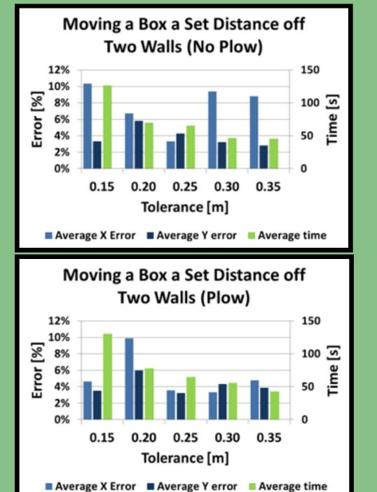
We were able to localize, push a box to a specified location, and dock with the robot. Performance was improved by adding a plow and refining the tolerance value.
