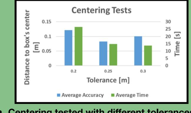
**Centering tested with different tolerances** (acceptable range of alignment accuracy) • Found that the optimal tolerance value is . 25 because it balances hardware and software error
