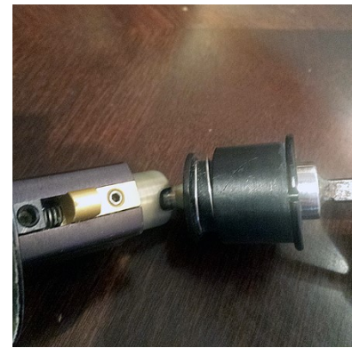
Figure 7.c. A dynamic extension of Brett's myoelectric prosthetic that can rotate with his wrist.
