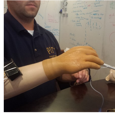
Figure 6.c. Brett demonstrating how he uses a paper clip and myoelectric arm to perform tasks as a nurse.
