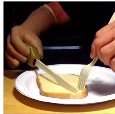
Figure 4.c. Brett slicing bread with his myoelectric arm and 3D printed knife holder.
