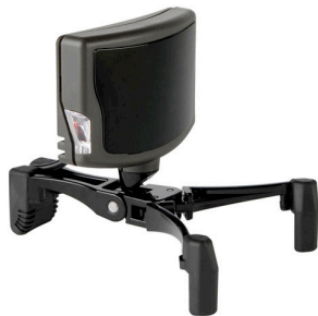
Fig. 1. NaturalPoint's TrackIR camera.
