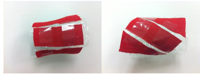
Fig. 3: Examples of low-fidelity prototypes created during the iterative design process; these two are made from plastic bottles, fabric, and tape.
