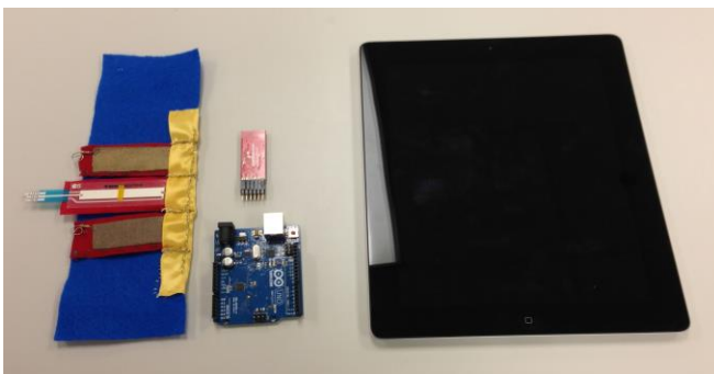
Figure 1: Our study materials included our wristband prototype, a Bluetooth modem, an Arduino board, and an iPad.
