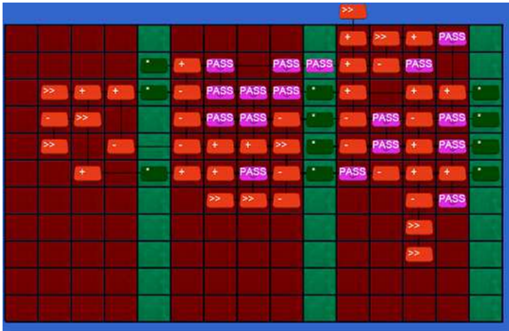
Figure 7 illustrating the prototype for the heterogeneous architecture a multiplier row is given at every 5 interval.
