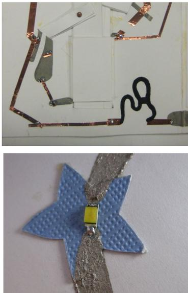
**Figure 2. Top: the back of one of our pages that includes conductive fabric (grey), resistive paint (black), and copper tape (orange). Bottom: an LED soldered to a trace painted in CuPro-Cote.**
