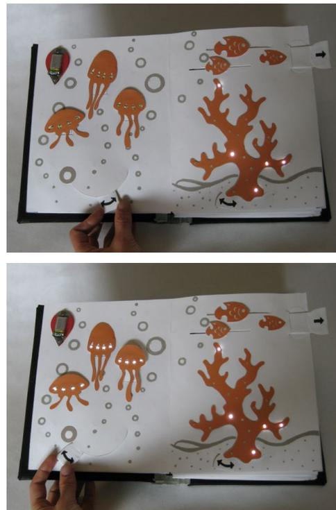
**Figure 5. Top: with the wiper to the left the jelly fish lights are off. Bottom: with the wiper to the right the lights are on. When the wiper is in the center of its track the lights are dim.**
