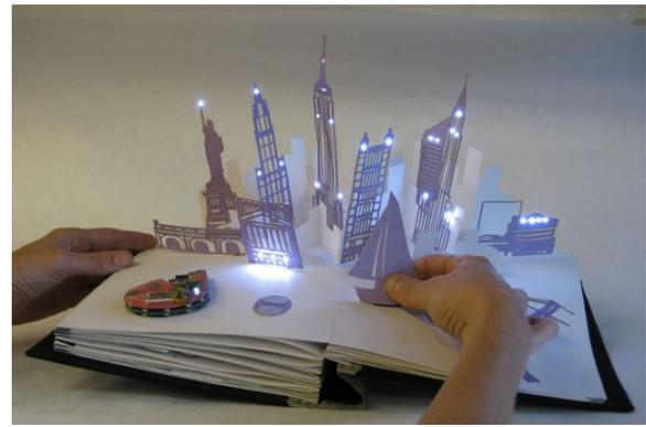
**Figure 11. A bend sensor (labeled with an arrow in the top image) controls the lights in the skyscrapers. In the top image the sensor is flat and only the bottom-most lights are on. In the bottom image, the sailboat is fully erect, causing all of the lights to shine.**
