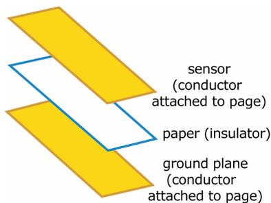
**Figure 14. A diagram of the capacitive sensor.**
