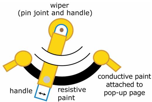
**Figure 7. The rotator potentiometer mechanism**
