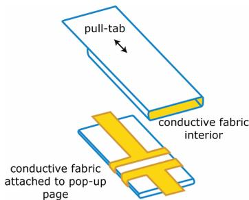
**Figure 5. A paper switch mechanism. Note: conductors are shown in yellow in this and all subsequent diagrams.**
