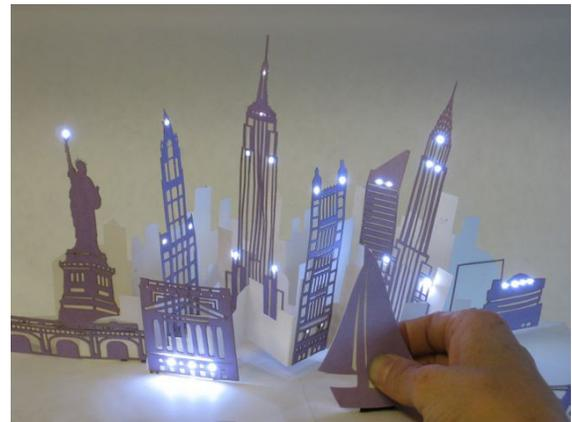
**Figure 1. A page from our book depicting the New York City skyline. A bend sensor—the flap in the shape of a boat in the foreground—controls the lights in the skyscrapers.**
