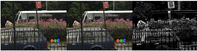
Fig. 4. The differences between two sequential frames in a video is shown in the third frame.
